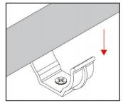
3)Open the pc clip, and put the lamp strip in a fixed position.
