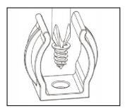
2)Adjust the pc clips to the proper position and use a screwdriver to drive the screw to secure it.
