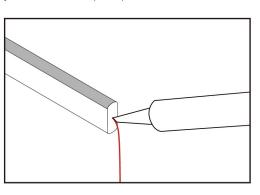
(3)Weld the positive and negative terminals to test whether the welding is correct
