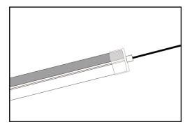
(4)Power test light attention to the positive and negative poles (If the lamp belt is not bright, the power interface is pulled out and the 180° reverse side is connected to the lamp belt)
