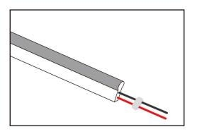
(3)Align the thick end of the pin with the power port and insert it firmly
