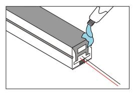
(2)Use tool to disassemble carefully, and do not pull the LED strip directly.
